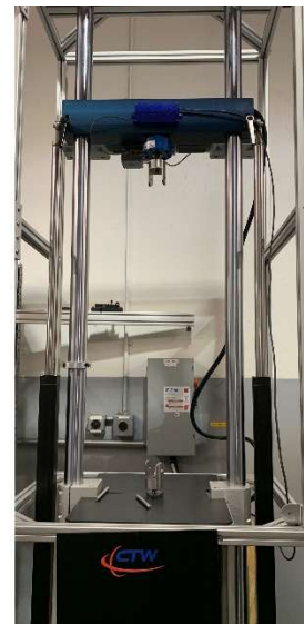
Complete LA with Automated crossbar and Enclosure showing full system and 1000 mm range of travel
