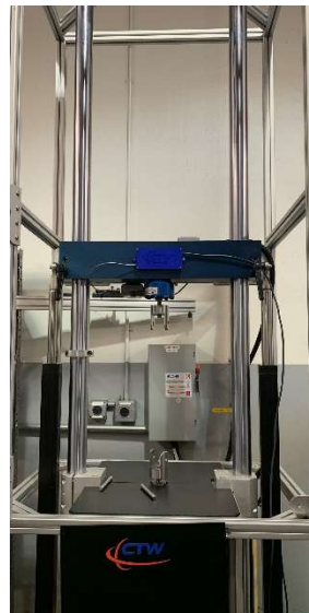
Complete LA with Automated crossbar and Enclosure showing full system and 1000 mm range of travel
