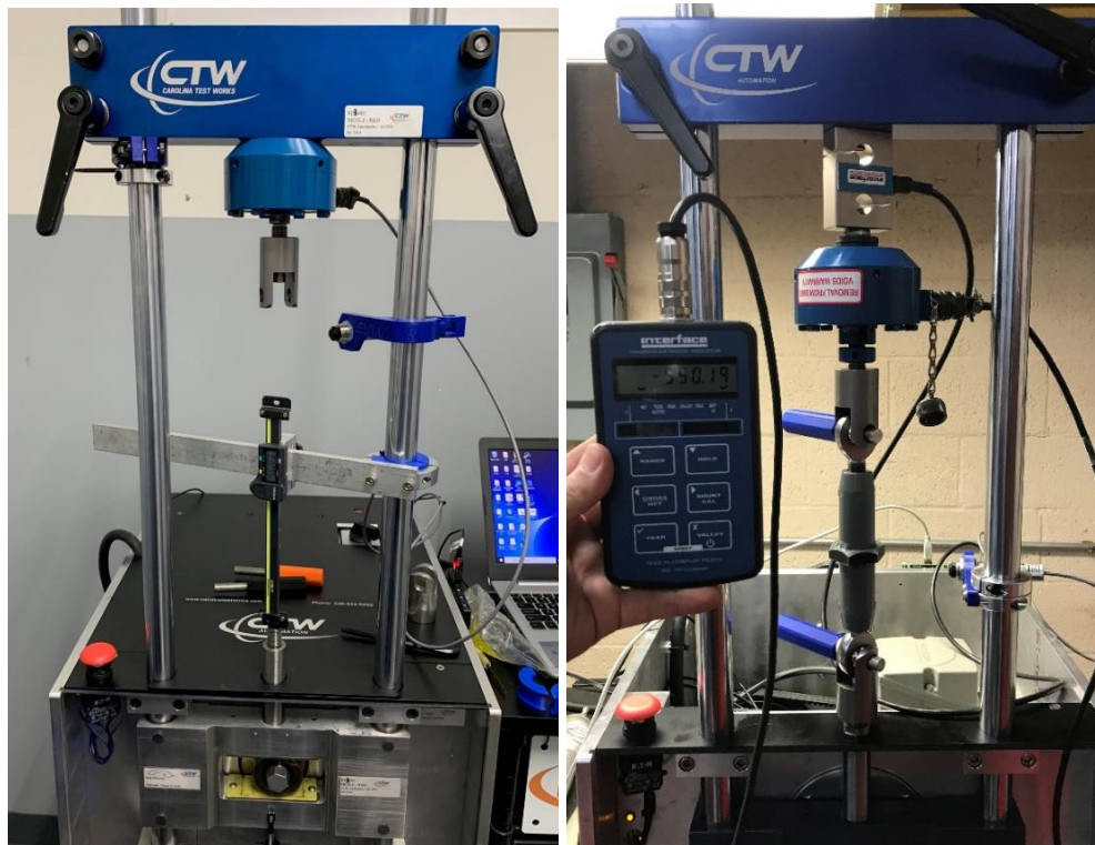
NIST Type Calibration: Displacement and Force signals
