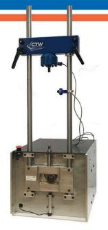
Computer controlled / variable speed / multi-channel data acquisition
