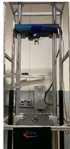
Complete LA with Automated crossbar and Enclosure showing full system and 1000 mm range of travel
