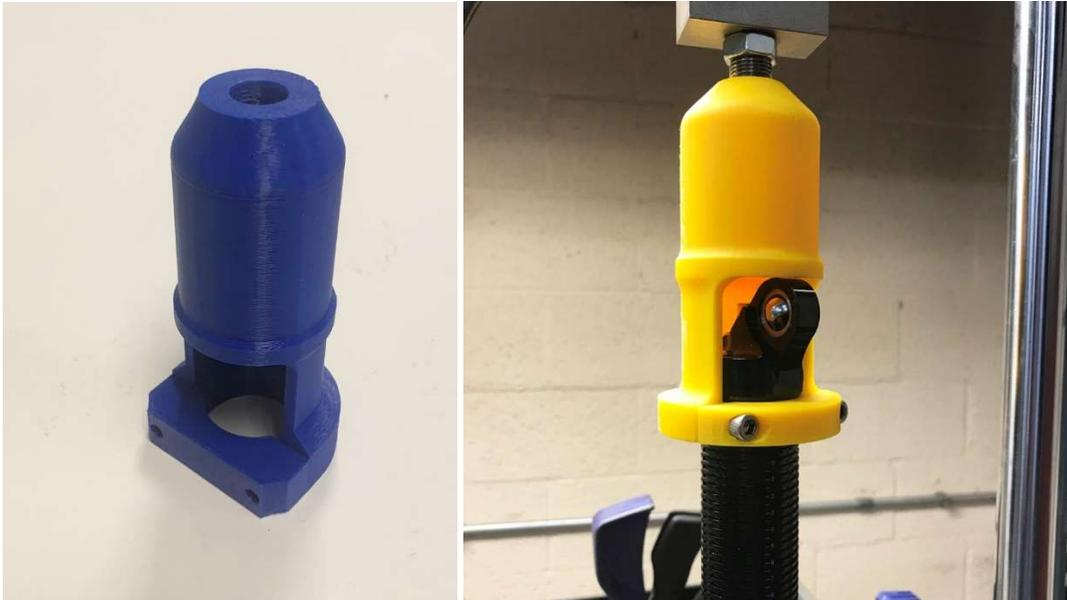
**Thru Rod Damper fixture – 3D Printed for ¼ Midget Dampers**
