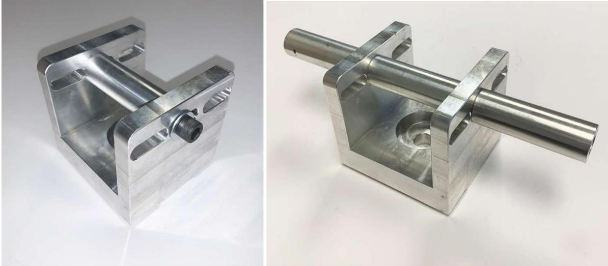
**Lower Fork fixture with single and dual mounting rods**
