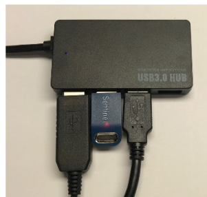
USB Hub with Software key – USB cable from Data card – USB for motor control
