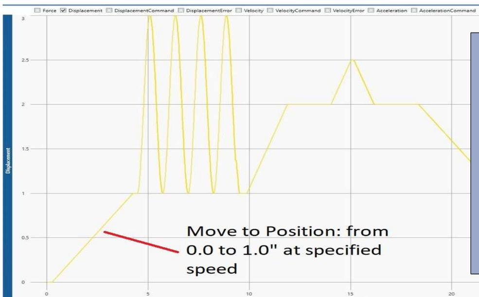
Example of the displacement trace of the beginning of a Test Sequence.
