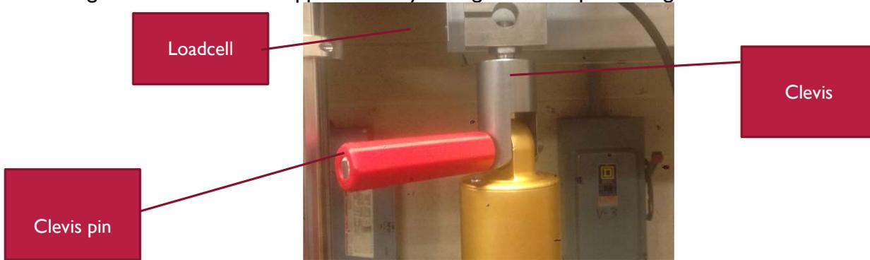
2. From the “test execution” page click the “zero force” button. This removes the weight of the shock or any offset in the loadcell out of the data.
