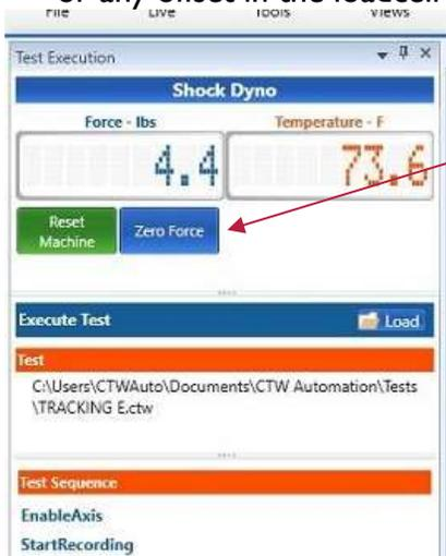
Zero Force – performs a tare of the load signal. You want to remove the weight of the damper and fixtures.
