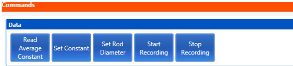
**Set rod diameter** - Select this button if you want to define your rod diameter and have the software save that number with the test. If a proper rod diameter is entered the software will record the gas pressure in the shock. This is based on the rod force recorded during a test (you must do a rod force test to get gas pressure).
