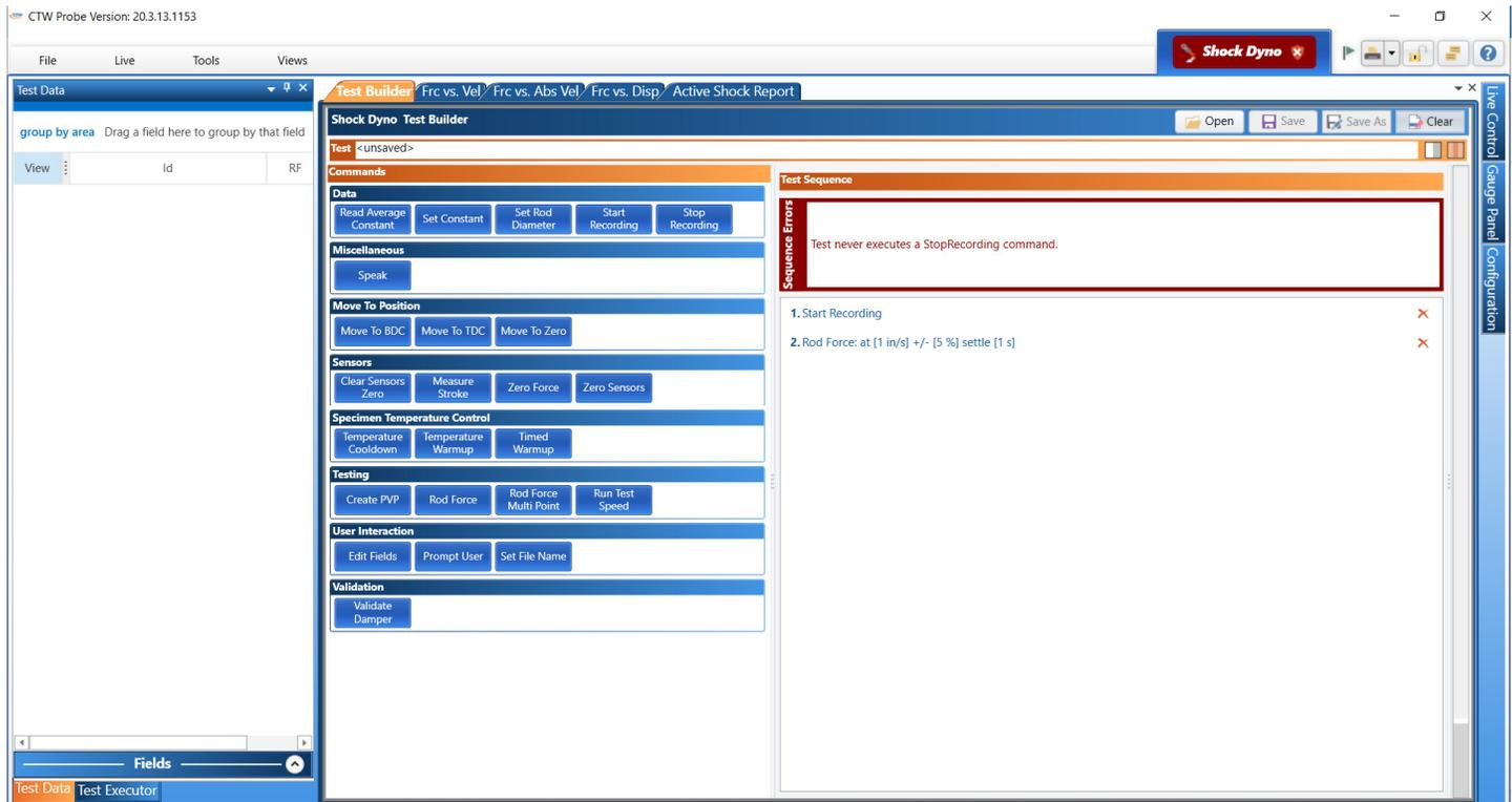
Clicking on the Test builder tab at the top of the page will open the window to create or modify a test. You can click on buttons to add steps to your test. When you click on a command in the “commands” column it adds that command to the “test sequence” column.
