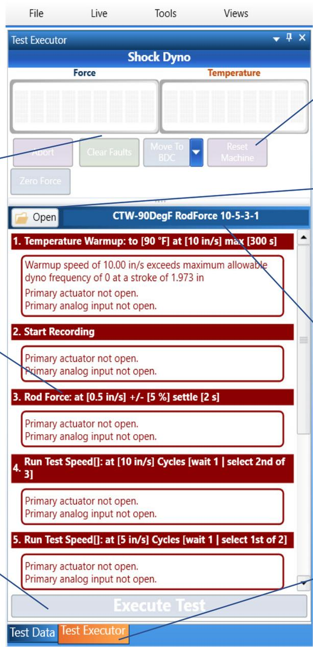
If command buttons are greyed out (inactive) that means there is a problem and test will not run, make sure power is turned on and all cable are connected
