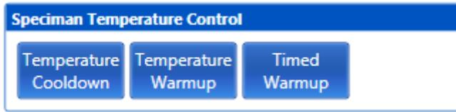
These buttons allow the user to warm the shock up before the test. You can warm up for a time or to a defined temperature. You can also run the shock slowly to allow it to cool down before removing. Once the button is selected and moved into the sequencer list double click on the button to open the parameters for that command.
