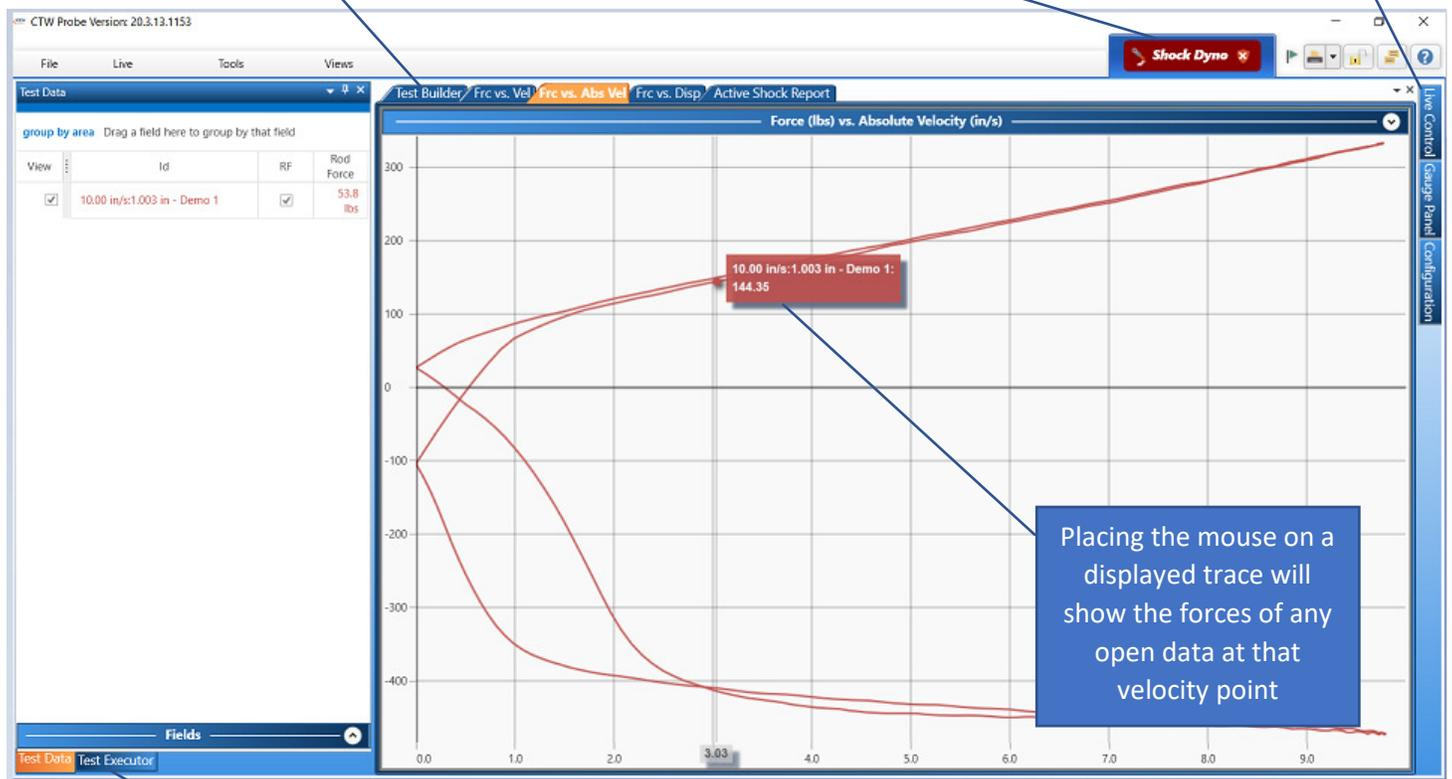
Placing the mouse on a displayed trace will show the forces of any open data at that velocity point
