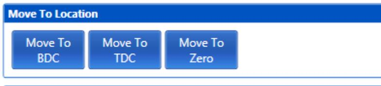
These buttons are used to tell the dyno where to park at the end of the test. For most users, select the Move to BDC button at the end of your test so the dyno will always return to the bottom of the stroke.
