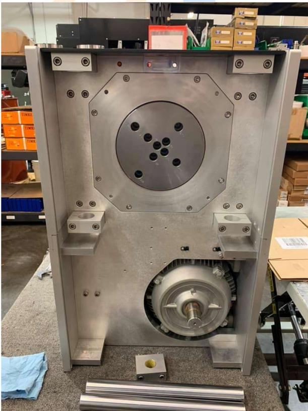
CTW has increased the peak available strokes of the RD7.5 and RD10. These new machines will have a peak stroke of 160mm. This will also increase the peak velocity up to 3.0 m/sec. Final specifications and performance will be added once we get the first one up and running.
