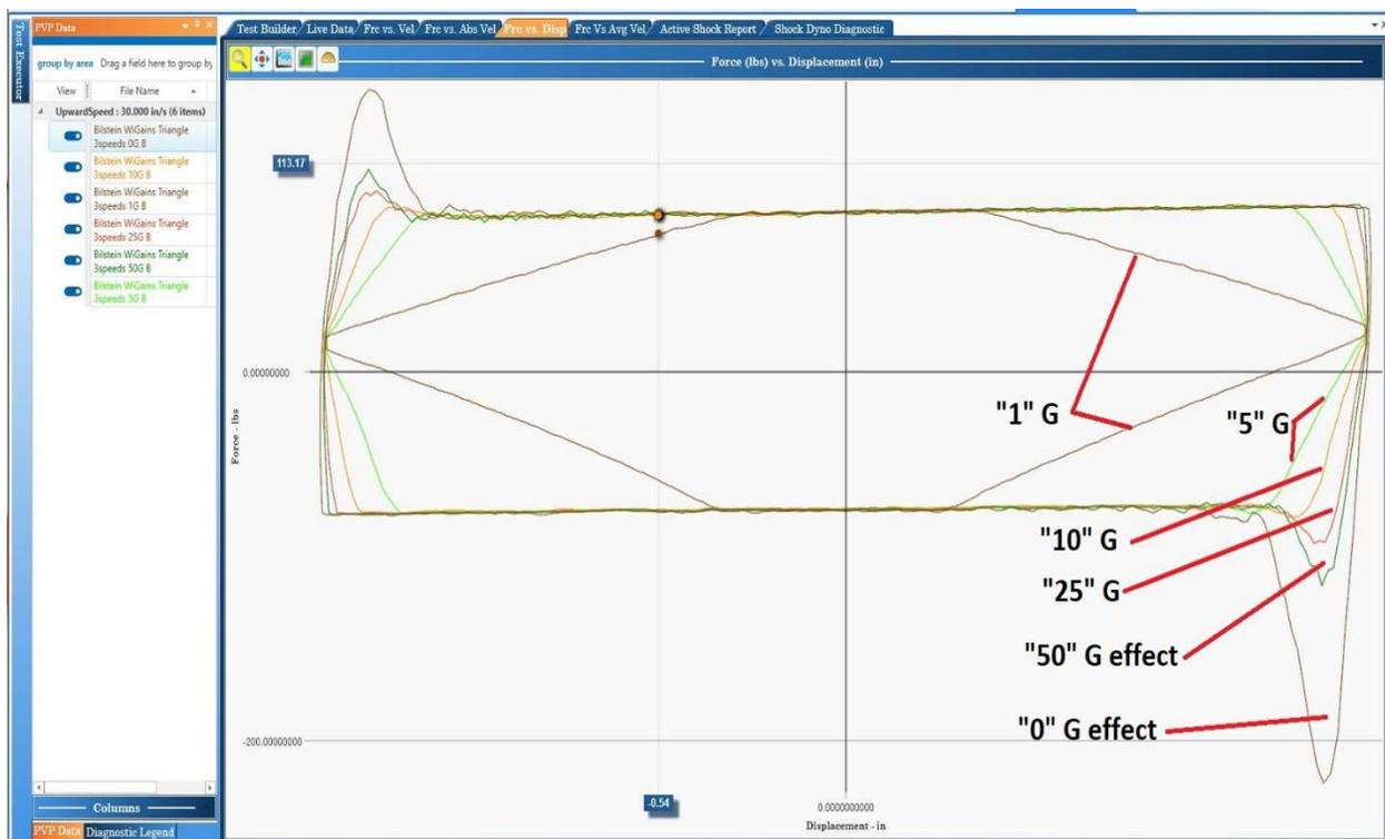
Force v Displacement from a series of Triangle waves
