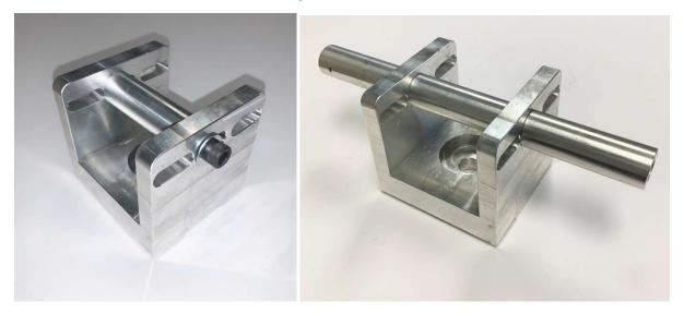
Lower Fork fixture with single and dual mounting rods
