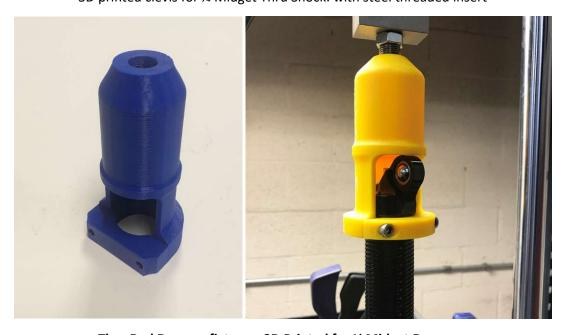
Thru Rod Damper fixture – 3D Printed for ¼ Midget Dampers
